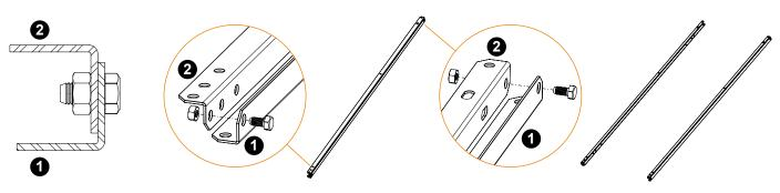
Place part 4 between the two Π shape parts constructed in the former step 1 in order for the frame to be formed. Screw straight parts 6 (which will be used for the mounting of the support base to the tiles) to the botton part. Repeat for the rest of the parts.
