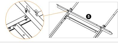
Bend the straight parts 6 of step 2 with the hand covering the beams of the tiled roof. Drill and fasten up with bolts. Use level so that the base is horizontally placed.
