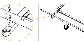
Screw the collector supporting part 5 to the top part of the frame without tightening the screws.
