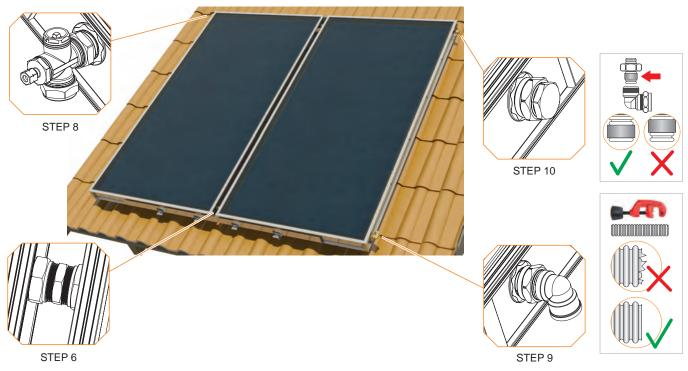
\*Use lock nuts in order to avoid the copper tube mechanical strain.
