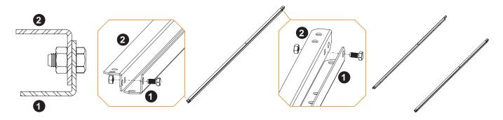
Place part 4 between the two Π shape parts constructed in the former step 1 in order for the frame to be formed. Screw straight parts 6 (which will be used for the mounting of the support base to the tiles) to the bottom part. Repeat for the rest of the parts.
