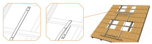
6. In case of two collectors, first place the left one, lifting the collector's upper and lower fixing washers 7. When the collector is placed under, we slightly tighten the M8 screws and nuts with the collector's fixing washers 7 in order to temporarily restrain it and easily center it with the system. Place the mechanically tightened unions Ø22 at the collector's edges.
